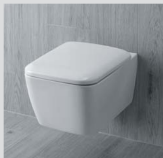
it! Wash-down WC, rimfree, 4.5 l/6 l, wall-hung, 350 x 540 mm, model no. 201950
